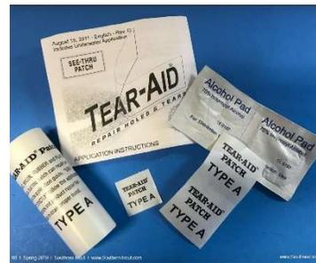
For a more significant tear, use a [Tear-Aid type A](#) patch for rubber, neoprene or breathable materials if the temperature is above 50°F. The patch should be one inch larger than the damage and be sure to round off the corners of the patch. A square edge
